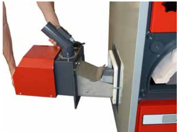
Burner removing for year servicing and cleaning
