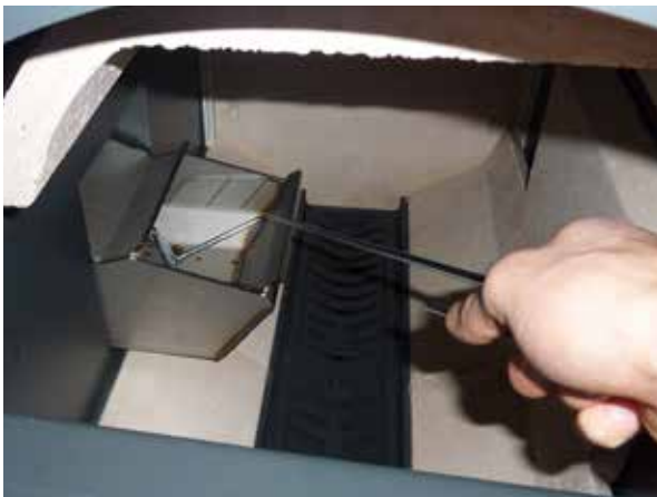
Cleaning of combustion chamber with fire hook
